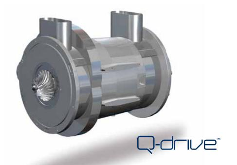
Quantima's  $^{\text{TM}}$  patented Q-drive  $^{\text{TM}}$  compression and motor assembly has just one moving part and operates with the rotor spinning in a magnetic field at up to 60,000 rpm.
